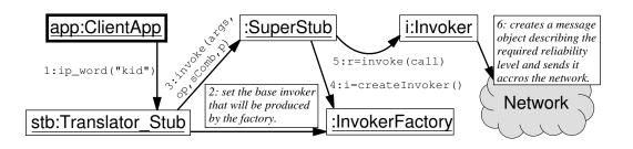
Figure 2: Partial view of the invocation path in the client side.
